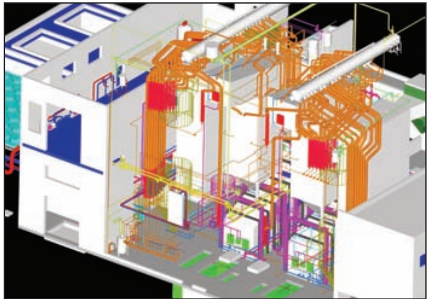
Designed with CADISON: 3D model of the biomass fired co-generation power station in the town of Bardejov in East Slovakia.
